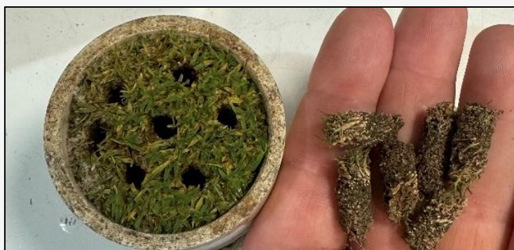
Thatch impact on Ksat is determined by coring samples in the lab.
